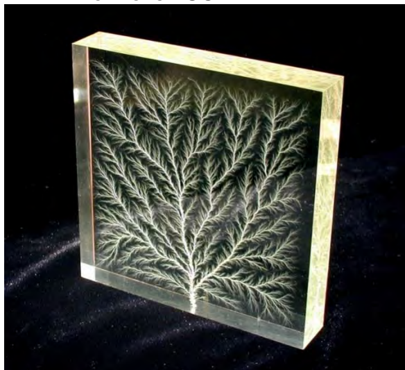
High-voltage breakdown within a 4 in (100 mm) block of acrylic glass creates a fractal Lichtenberg figure
